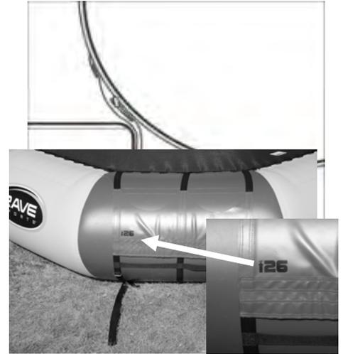
Position all three ladder buckles so they are directly over the inside seam line of your RAVE product as shown. NOTE: This is critical for the secure/safe mounting of the Water Whoosh to your RAVE inflatable.
