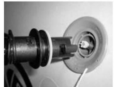
If you are using the RAVE Sports High Speed Inflator (*Item #01083*), simply lock the adaptor onto the end of the inflation hose and insert into the valve body. Turn  $\frac{1}{4}$  turn to lock in place.
