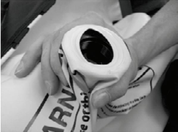
After the valve is cracked loose from the inflatable tube, you should be able to unscrew it the rest of the way by hand. When removing the outer valve body, ensure you maintain the position of the inner nut portion with respect to the hole in the fabric. Continue to hold tight onto the inner nut portion of the valve and do not allow the nut to move inside the tube or it will be very difficult to reposition it when installing the new valve.
