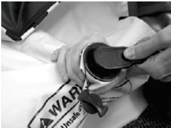
After the valve is out visually check the inner nut to be sure that it is not cracked or damaged. If not, simply screw in the new valve by hand. Be careful when starting the new valve into the nut to ensure the valve and nut are not cross threaded.
